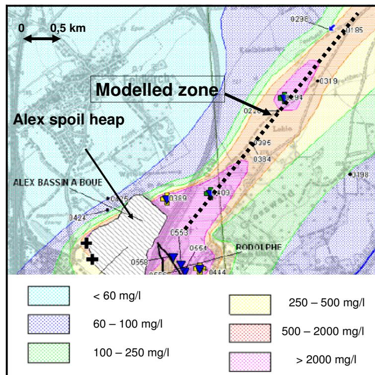
Figure 3. A chloride pollution map of the modelled zone, downstream from the spoil heap Alex.
