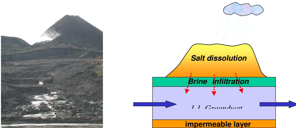
Figure 2. Picture of a potash mine spoil heap, and scheme of brine infiltration into groundwater.
