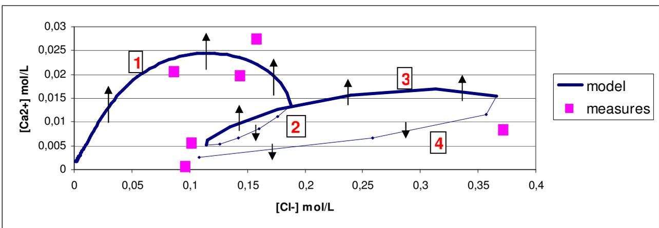
Figure 5. Calcium concentration versus chloride concentration downstream from spoil heap Alex.
