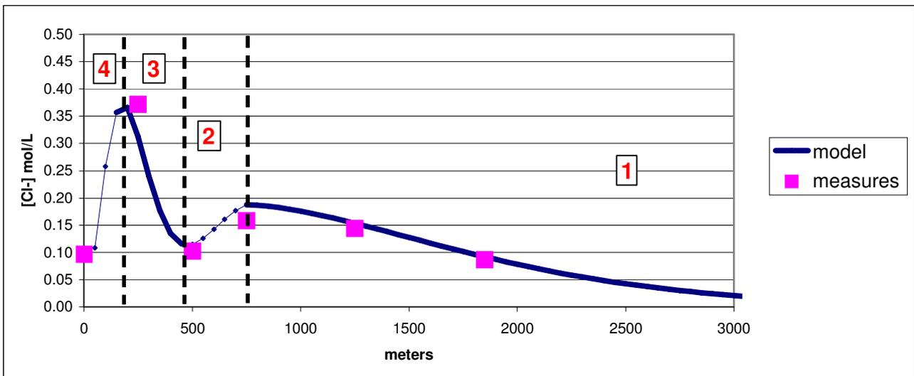
Figure 4. Spatial distribution of chloride concentration downstream from spoil heap Alex corresponding to the different stages of pollution: (1) 1910-1976 ; (2) 1977-1989 ; (3) 1990-2001 ; (4) 2002-2005.
